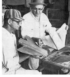
SANDIA'S FOUNDRY made a sand casting from the wooden model—in this case, the wings and part of the fuselage. D. A. Quayle (left) and C. C. Riley (both 4221-2) are checking the almag casting against the pattern.
